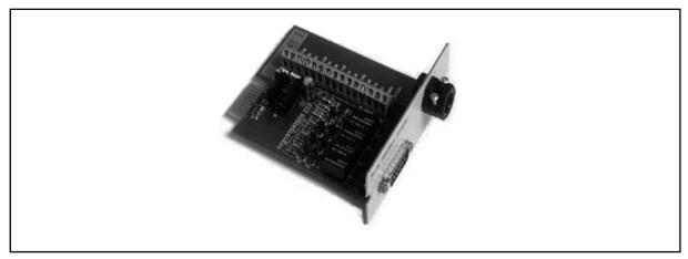
Figure 14 AS400 Relay Module.
